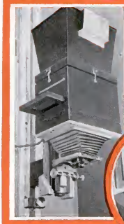
This homemade enlarger runs on a tongued-and-grooved slide, fastened to the wall. The focusing is done by means of two small pulleys and fishline
